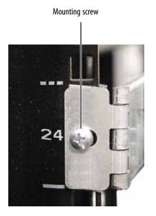
8 Align the mounting screw holes in the server handles with the front mounting nuts, then secure the front in place with two mounting screws (one on each side).
